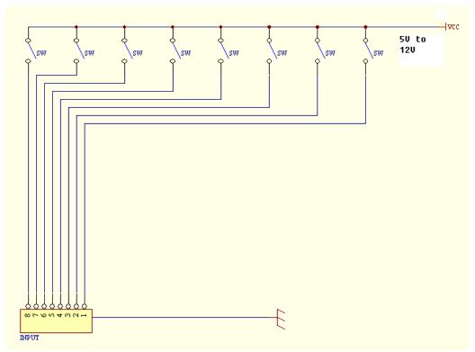
**Example of Trigger Input Connections**
