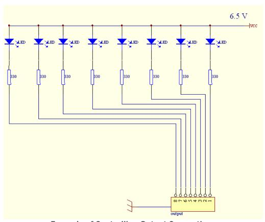
**Example of Controlling Output Connections**
