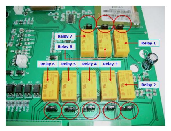
To set the output relays to dry contact when activated, please adjust the jumper according to the below diagram
